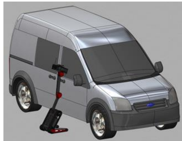
Figure 3 - Example of the long reach capability the Mark IV was designed to achieve. Robot pictured is the Servosila "Engineer". Source: https://www.servosila.com/en/mobile-robots/index.shtml
